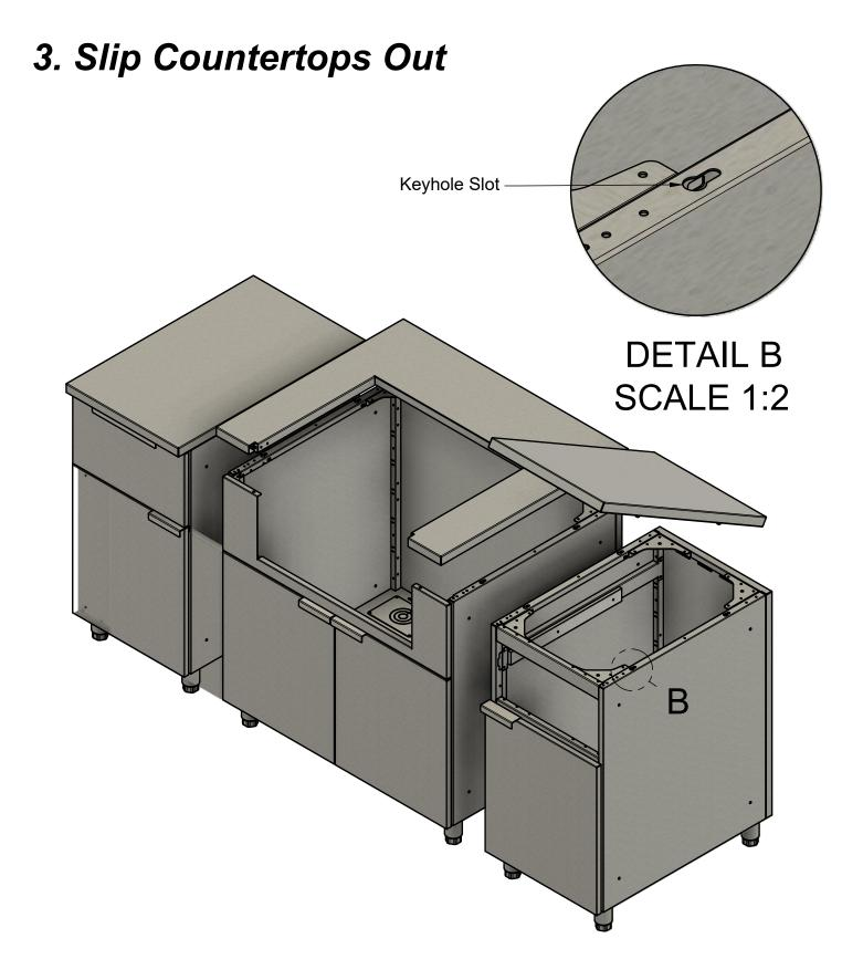
With the countertop screws loosened off, pull the countertop forward towards the front of the cabinet.
