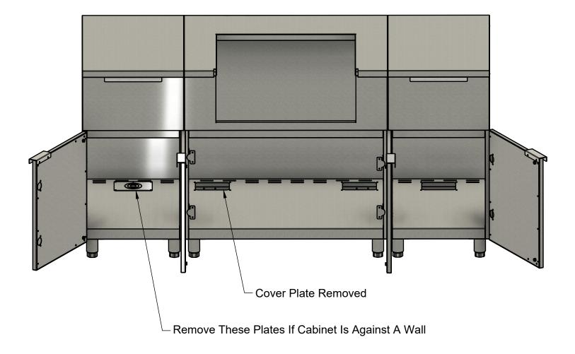
The cabinet assembly should be leveled in its final position for best results, and re-leveled if moved.
