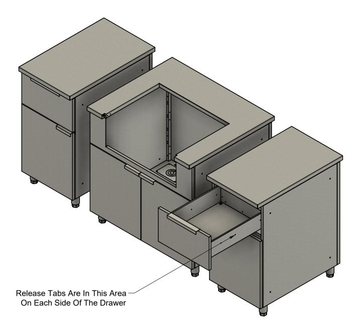
Remove any top drawers to access the screws holding the countertops in place.
