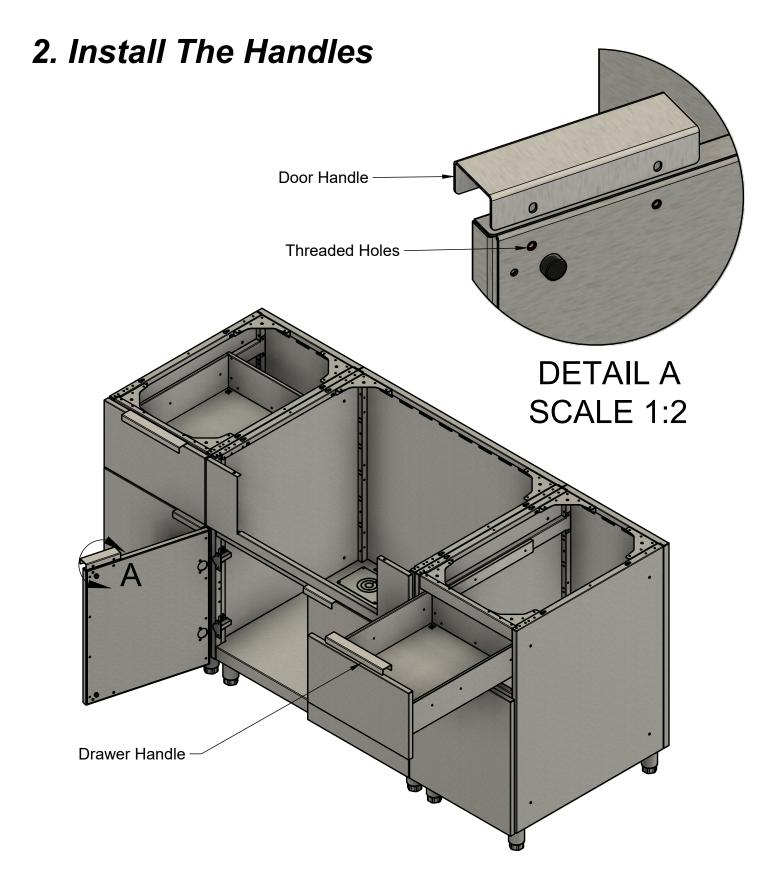
Install the drawer and door handles by slipping them over the door or drawer, and attaching them using (2) of the provided 8-32 button head screws through the handle into the threaded holes.
