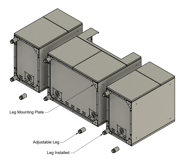
Flip the cabinets onto their backs, onto a moving blanket or other scratch free, soft material.
